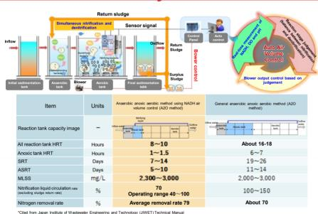
▲ Reduced reaction tank staying time and nitrification liquid circulation rate
