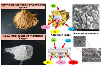
The schwertmannite system insolubilizer with iron as the main material, and the hydrotalcite insolubilizer with aluminum and magnesium as the main materials Anions are drawn inside, and cations are adsorbed on the surface.
