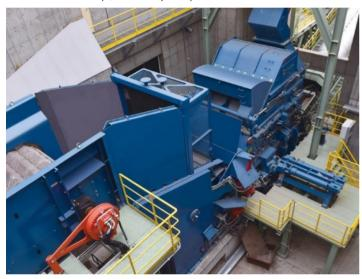
Mixed metal continuous sorter A device that can separate metals with specific gravity by fluidizing power sending air from the bottom of filled powder.
