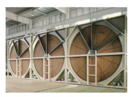
▲ VOC concentrated rotor. Hydrophobic zeolite supports inorganic honevcomb.
