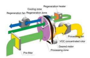
▲ When exhaust containing VOC passes, the VOC is adsorbed and concentrated on the rotor surface. By passing a small amount of hot air, this can be recovered as high-concentration VOC gas.
