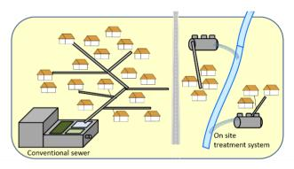
Proposed septic tank implementation plan in combination with existing sewage treatment facilities
