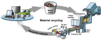
▼ Illustration of identification using Raman spectroscopy
