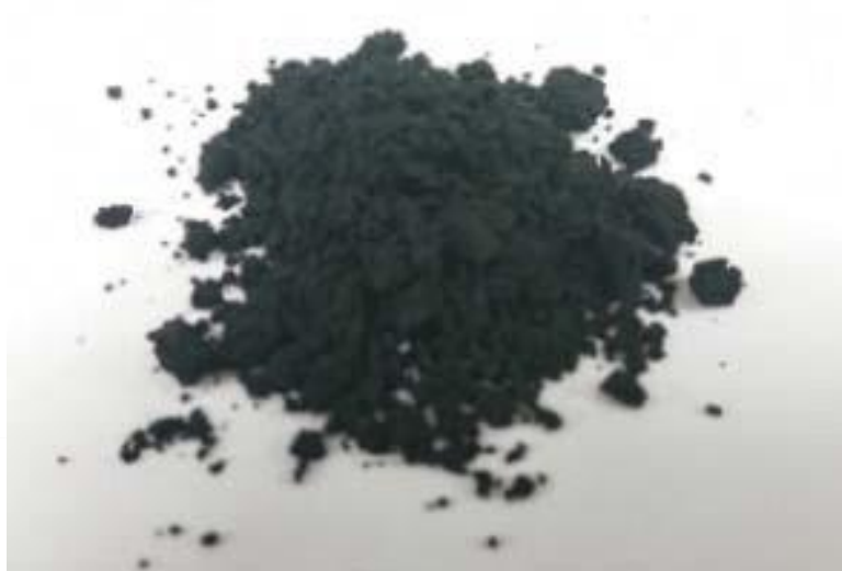
▲ Appearance of Catalyst BP. A moist black powder that disperses well in water
